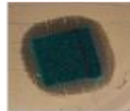
Inhibition halo test of POLITO coating on cotton
